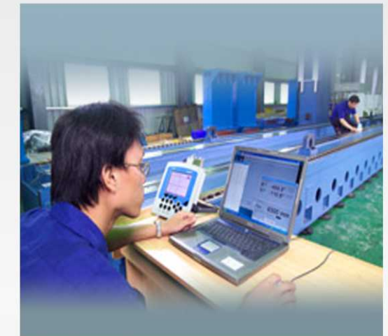
Max. measurement travel 20 m. Straightness is inspected by optical instruments.
